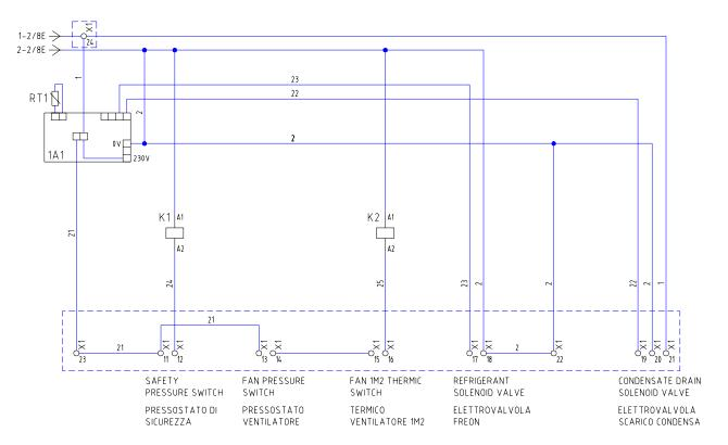
G5C 250 (460/3/60) CONTROL WIRING DIAGRAM - Cod. 714.003.02.00 - Rev. 03 - 02.05.02
